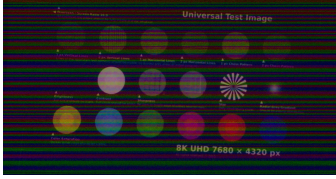
Fig. 5. Image with 10mV noise (No LDO)
