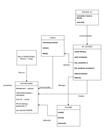
Fig. 1. UML diagram of our classes
