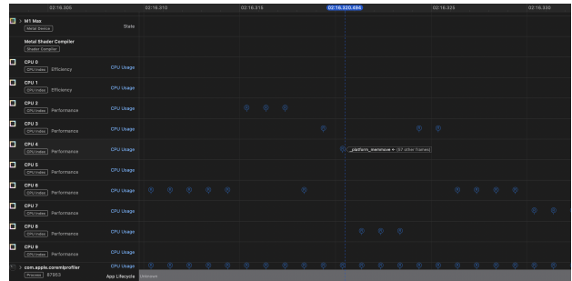
Fig. 17. Zoomed in Core ML instrument for 'text encoder' showing the distribution of operations between cores.
